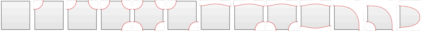
Fig. 5. The 13 configurations of patches (all of them sub-rectangular) that can occur in our free-boundary motorcycle graph. Arcs are depicted in black, boundary segments in red. The depicted shape of the red boundary segments is exemplary and can vary – to some extent, as long as it does not form any concave peaks in the interior.
