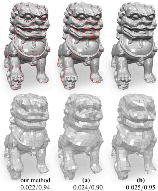
Figure 11: Comparison of our scale conforming FCN as guiding constraints for quadmeshing to constraints induced by setting curvature thresholds as in [BZK09]. The top row depicts the guiding constraints. We choose a high curvature threshold in (a) to preserve only strong features and avoid degeneracies in the parametrization. If this threshold is increased in (b) nearly all strong features are removed simultaneously. The numbers below give the Hd/average Scaled Jacobian (aSJ). While in (a) the quads align along the features the aSJ is much lower than in (b), which has a high aSJ due to the low number of constraints, but quads do not align well along features. We can observe that the aSJ is similar to that of (b), while still aligning well to the features at the given scale.
