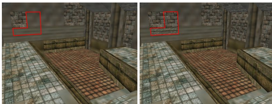
Figure 4.2: Example of a so called LOD Snap . A low resolution page is exchanged by its high quality counterpart within the course of one frame.
