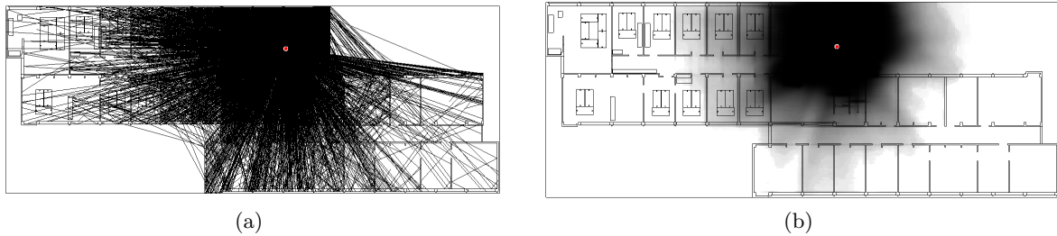
Figure 1: (a) A sparsely sampled Photon Path Map in an indoor scenario. (b) The same map, more densely sampled and with the field strength coded by using grey scales. In the black areas the field strength is high, whereas transparent or white areas have low field strength. Both images represent the top view of a 3D simulation.
