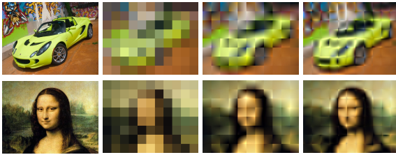
Figure 5: The approximation quality of our image descriptors on two examples. From left to right: original image, constant, bi-linear and bi-quadratic approximation. In all cases 8 \cdot 11 tiles were used.
