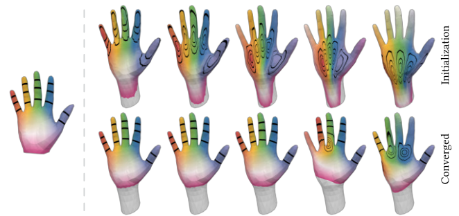
Fig. 11. We compute maps between two hands, starting from increasingly challenging initial maps (top row). Our optimization (bottom row) recovers the expected map as long as the initialization is reasonably close.
