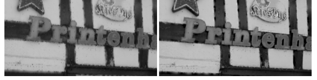
Figure 2: Left: Intensity Completion preserves intensities and varies the gradients between projected points as little as possible. Right: Gradient Completion additionally preserves intensity gradients taken from the reference image resulting in visually much sharper image features leading to more accurate SIFT descriptors as shown in the results.
