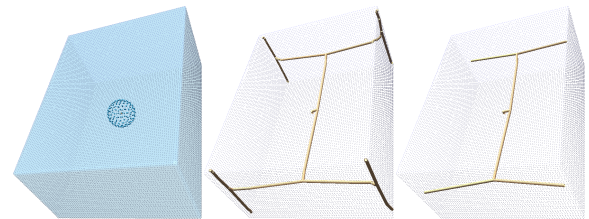
Figure 6: The result of our algorithm is a thin, 1D curve-skeleton even in degenerated cases such as a 3D box. When the initial model is not exactly centered (left), the skeleton quickly recovers the symmetry of the input (center). The filtering preserves the symmetry (right).
