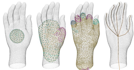
Figure 2: The deformable model with competing fronts. The fronts move in a coarse to fine manner; and may split to form sub-fronts, inducing the branching structure of our skeleton.
