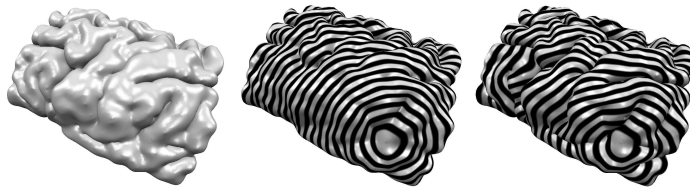
Fig. 6. Geodesic distances. For visualization purposes the geodesic distances are color-coded as black and white stripes. Left: Reconstruction of a part of the cortical surface. Middle: Without topology control the sulci are not correctly reconstructed. Right: Using topology control the distance field correctly follows the sulci and gyri.
