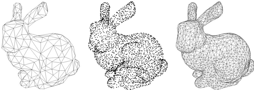
Figure 1: In order to avoid that the robust transmission becomes as complicated as the general surface reconstruction problem from point clouds, the sender (who knows the original mesh) provides additional information to the receiver which simplifies the reconstruction ( hinted reconstruction ). In this case the sender provides a coarse base mesh to convey the global surface topology. All other mesh vertices are sent without any connectivity information. The receiver can approximately reconstruct the original shape by inserting the vertices into the mesh based on spatial proximity.
