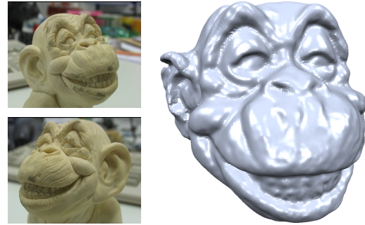
Figure 7. Reconstruction from low-quality images. Left: First and last image of the input sequence. Right: triangle mesh.
