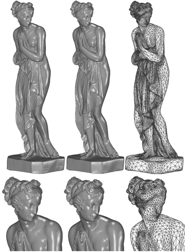
Figure 1. Original Iphigenie model (left): scanned data 351750 points, Loop surface approximation (center): maximum deviation is 0.05% of the bounding box diagonal, control mesh defining the surface (right): 15347 control points.
