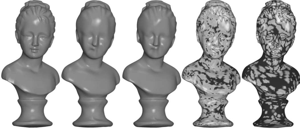
Figure 3. From left to right: a) original model with 30696 sample points, b) initial approximation with 461 control points, L^2 error 82.9, c) after 25 parameter correction and re-fitting steps, L^2 error 42.6, d) and e) show color coded errors before and after the 25 optimization steps. Notice the concentration of the error to local “hot spots” which makes it easier to detect regions where the insertion of new control vertices effectively reduces the L^\infty error.
