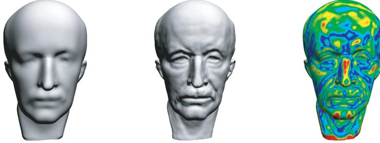
Fig. 2. Multiscale encoding: The point cloud in the middle is obtained as a normal displacement of the point cloud on the left. The right image shows the corresponding detail coefficients, where blue indicates maximum negative displacement and red maximum positive displacement for outward pointing normals.
